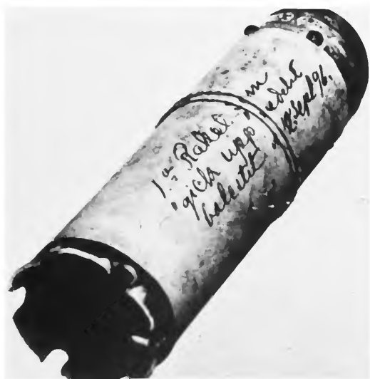
FIGURE 5.—The first known ballistite rocket, fired 12 September 1896 in Stockholm. In Tekniska Museet, Stockholm.
