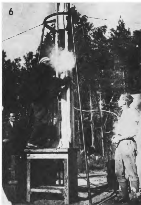
FIGURE 6.—Loading a Rocket 09 with liquid oxygen.
