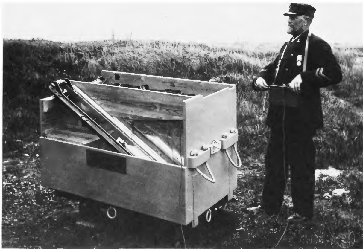
FIGURE 10.—Complete lifesaving rocket system, manufactured by the Mars Company. Photo from Armémuseum Archives, Sweden.
