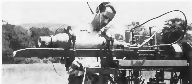
FIGURE 18.—H. F. Pierce making final adjustments preparatory to testing a large liquid-propellant motor, designed and constructed by Alfred Africano, on the ARS No. 3 proving stand on 22 June 1941.
