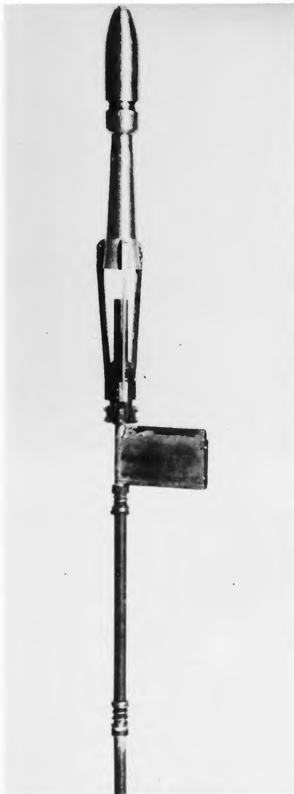
FIGURE 3.—Multiple-firing, solid propellant rocket. Cartridges contained in magazine at center are propelled forward by gas pressure into firing chamber resulting in repeating, intermittent thrust.
