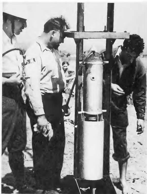
FIGURE 9.—ARS Rocket No. 3, at Marine Park for launch attempt in September 1934. From left, Shesta, Pendray, and Smith. The gasoline tank is being pressurized with nitrogen through a valve in the cone. The oxygen fill-hole is visible just below the pressure inlet. Photo from Pendray Collection, Princeton University Library.
