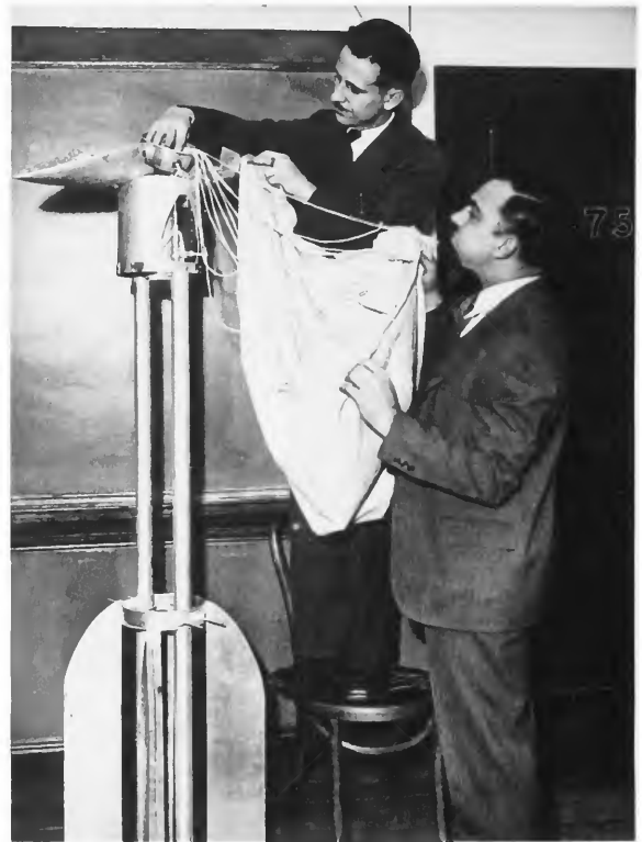
FIGURE 2.—ARS No. 1, during a demonstration and lecture at New York University (Washington Square Campus), in spring 1932. Hugh F. Pierce, who constructed the rocket, is packing the parachute in its container (made from a ten-cent-store saucepan) as G. Edward Pendray, co-designer of the rocket, holds the parachute. The cone-shaped nose was designed to open up at the height of the flight and eject the parachute. The parachute itself, made by Mrs. Leatrice M. Pendray from a scaled-down design for a professional aviation parachute, was of silk pongee. Photo from Pendray Collection, Princeton University Library.
