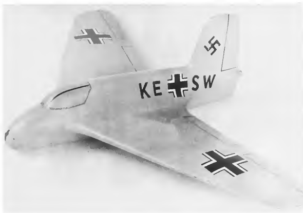
FIGURE 1.—Model of DFS-194, a further development of the DFS-39 which was flown by R. Opitz without engine in 1937. The next model, DFS-40, since the H_2O_2 rocket engine was not ready yet, was equipped with an Argus aircraft engine in 1938 and flown by H. Dittmar. The follow-on, DFS-194, was flown by H. Dittmar in the winter of 1938–39 and became the forerunner of the Me 163. Alexander Lipisch was the designer of all of these planes. Photo courtesy R. Opitz.
